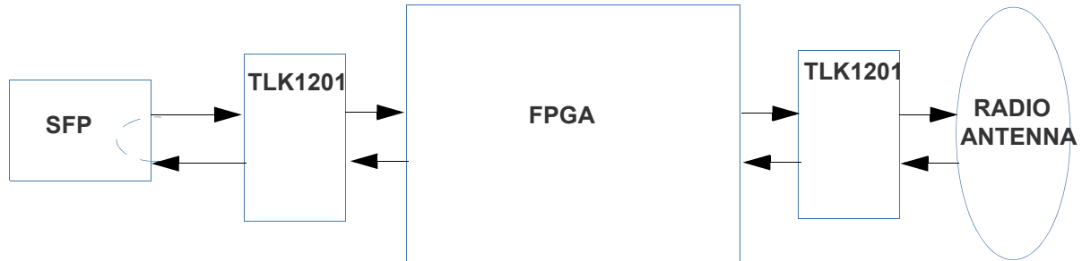
Figure 7-14 Radio to SFP Local Loopback path.
