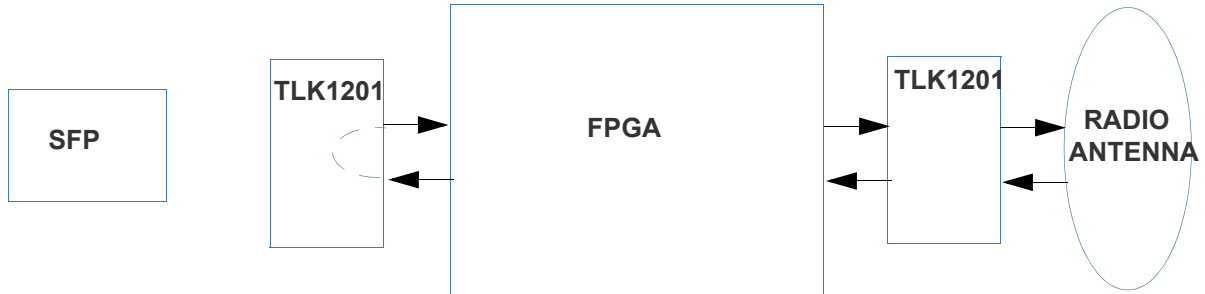
Figure 7-11 Radio External Loopback / Customer Local Loopback Configuration.
