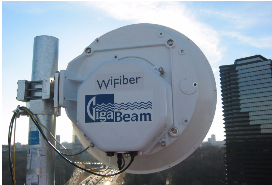
Figure 1-1 WiFiber G1.25 millimeter wave radio.
